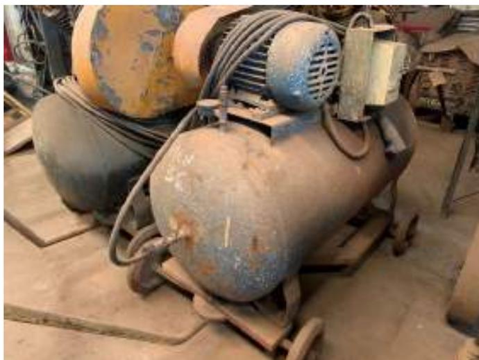
Item 37.a: COMPRESSOR DE AR COMPRIMIDO - MARCA SCHUZ - 20 PES, MOD. C149505, PRESSÃO MÁXIMA 13,50 BAR, MOTOR ELETR.TRIF.WEG, MOD 132M-1175 5CV 1740 RPM
